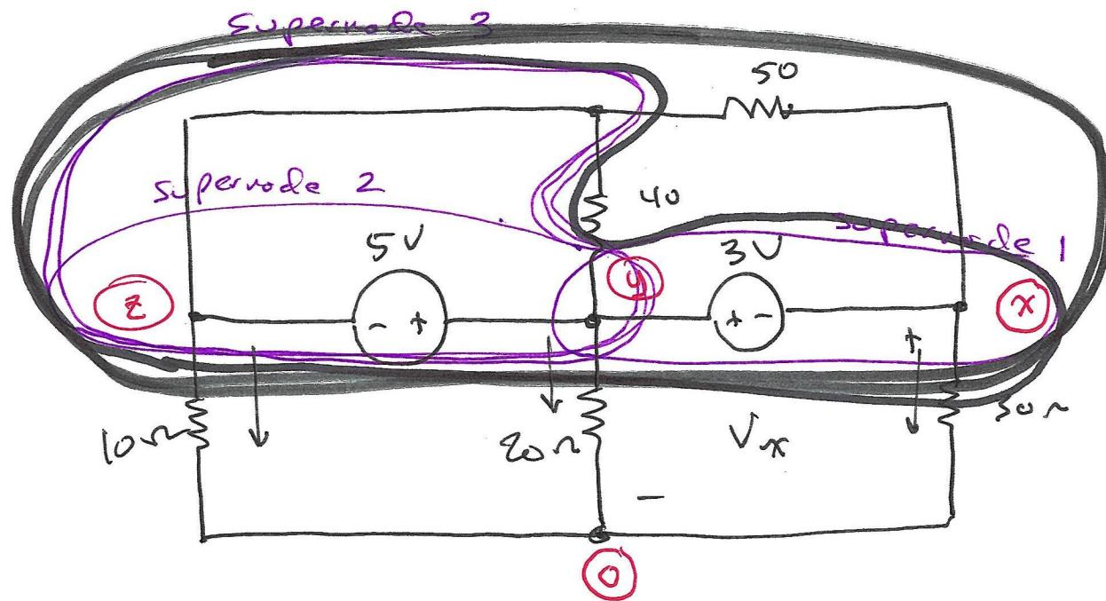
$$V_y - V_x = 3 \quad (\text{constraint eqn. for supernode 1})$$
