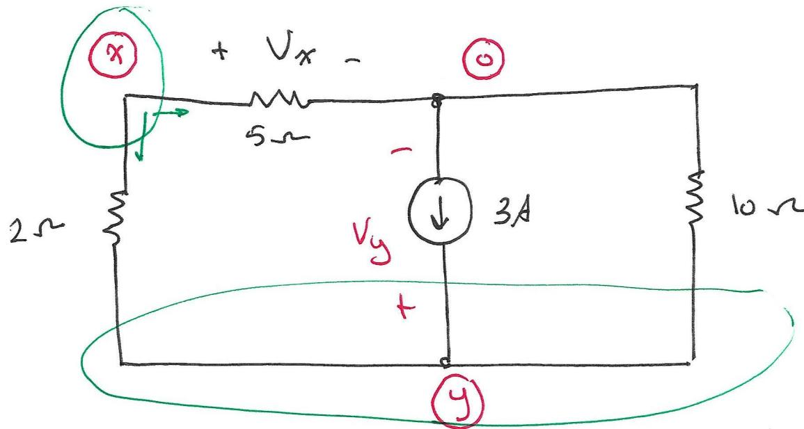
$$\frac{V_x}{5} + \frac{V_x - V_y}{2} = 0 \quad \text{at node } x$$
